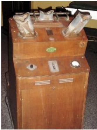
A shoe fluoroscope at the US National Museum of Health and Medicine. Public Domain. CC by J. S. Ballard
