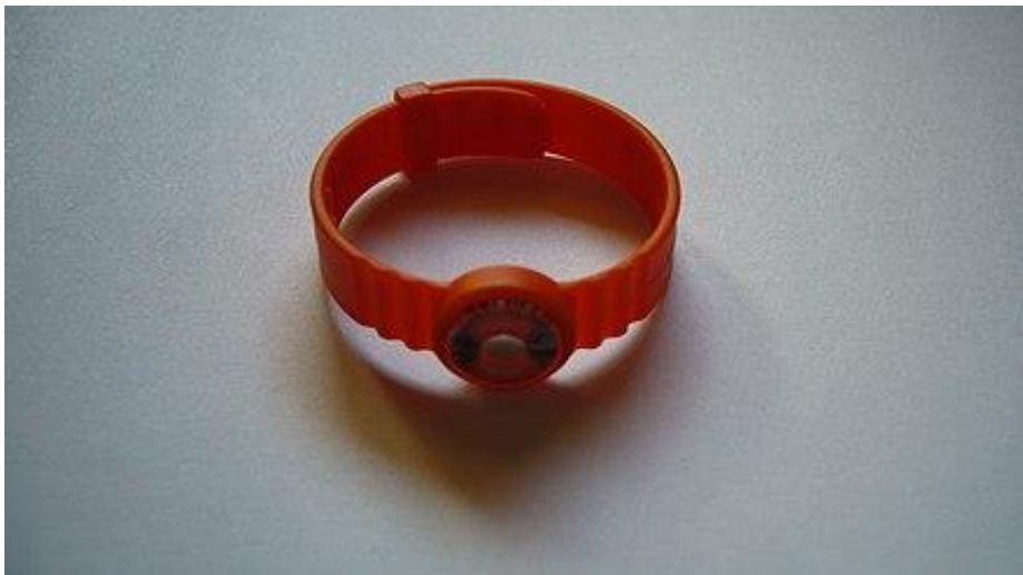
(TLD ring Wikipedia contributors, 2024 public domain Thermoluminescence dosimeter in the form of a finger ring for measuring radiation exposure to fingers and hands
